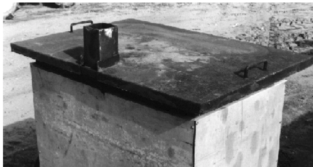
Photo 15. Wax dipping unit with lid in place.
