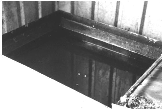
Photo 7. A vat of molten wax ready for dipping of hive material. Note: Hot wax dipping should not be done in an enclosed space. The owner of this vat plans to increase the head space between the surface of the wax and the rim of the vat. This will improve the safety margin in case of a boil over (refer to section on vats).
