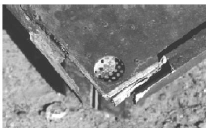
Photos 2 and 3. Examples of wood decay in a clearer board (left) and hive (right).
