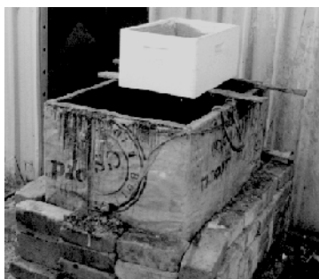
Photo 16. This vat is capable of dipping four supers at a time. Supers are removed from the wax and placed on two metal cross beams to allow excess wax to drain. The vat is partially insulated with aluminium sisalation and bricks. Completion of the brickwork would greatly improve the insulation and prevent heat loss.
