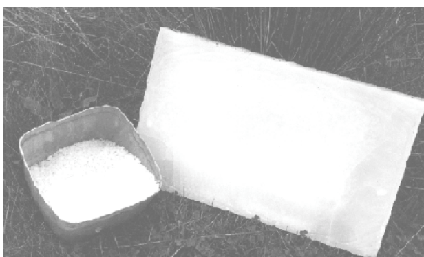
Photo 4. Microcrystalline beads (or pastilles) (left) and block of paraffin (right).
