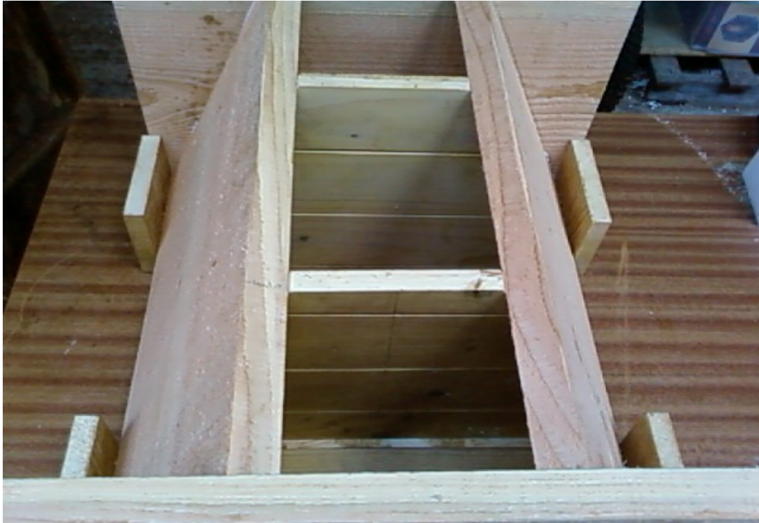
Showing the use of the jig to keep the sides in position.
